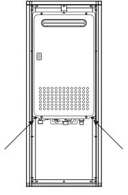
Figure 4: Location of lower mounting brackets.
