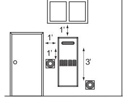
Figure 1: Discharge Vent Clearances.
